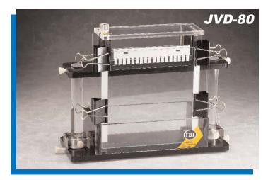
**JVD-80 comes complete with:** upper and lower reservoirs, two inner glass plates, two outer glass plates, 16cm support rods, two 1.5mm  $\propto$  18 tooth combs, two 1.5mm spacer set, four spacer tabs, safety covers, eight sandwich clips, power cords, and operation manual.
