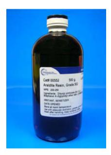
WPE is <u>Weight Per Epoxide</u> equivalent. From this value, one determines the optimum amount of DDSA or NMA in grams to combine with 100 grams of resin for stoichiometric balance minimizing unreacted starting materials and producing reproducibly stainable, embedding blocks.
