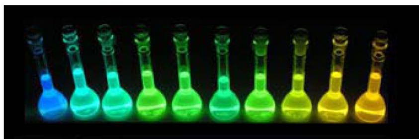
Fig1. Emission spectra change of solvatochromic fluorophore
