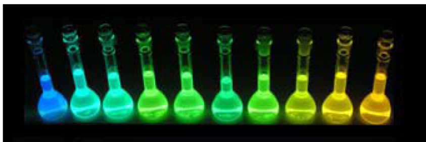
Fig1. Emission spectra change of solvatochromic fluorophore
