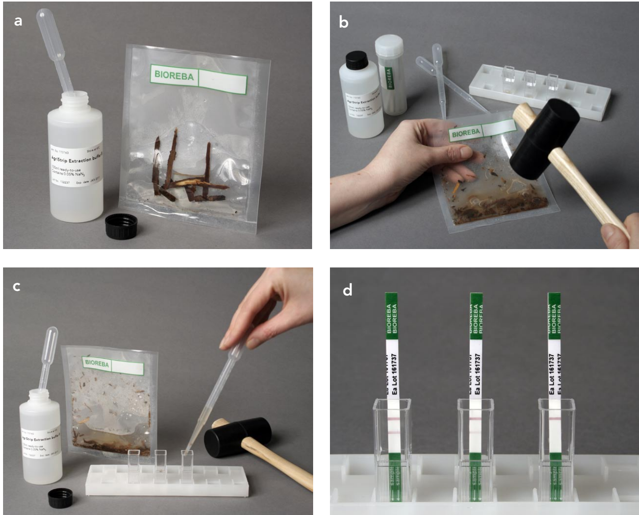
Fig. 3. AgriStrip Test procedure
